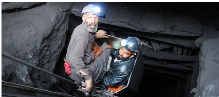
Figure 4. Metallic trolleys pulled and cables system for transportation of coal miners
