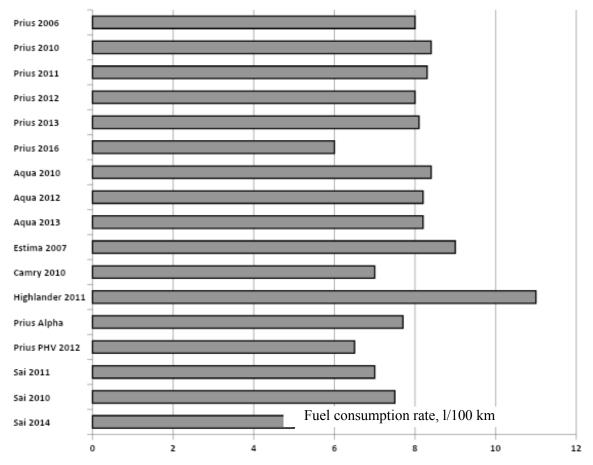
Figure 2. Fuel consumption rate depending on the Toyota cars year of manufacture.
