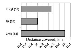
Figure 5. Curve of the distance covered at one fuel liter in relation of a Honda average velocity.
