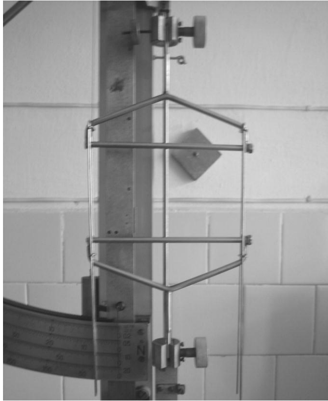
Figure 2. - Appearance of special device for research deformation behaviors of the high-elastic materials
