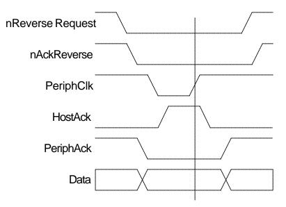
Figure 4. Enhanced Capabilities Port Reverse Command Cycle.
