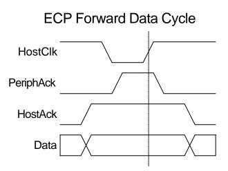
Figure 1. Enhanced Capabilities Port Forward Data Cycle.
