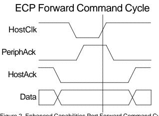
Figure 2. Enhanced Capabilities Port Forward Command Cycle.
