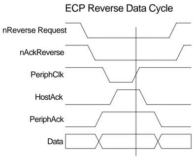
Figure 3. Enhanced Capabilities Port Reverse Data Cycle.
