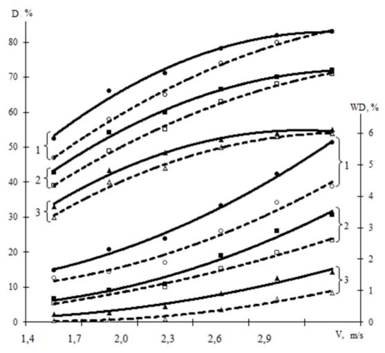
**Figure.1** Influence of the movement speed of the units and the width of the protective zone on the weed destruction degree (WD) and damage to soybean plants (D) during inter-row processing of belt-free crops.
