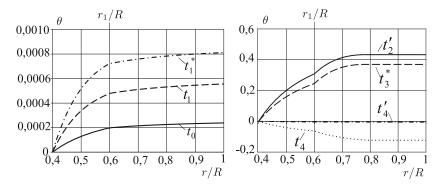
Fig. 3. Distribution of the rotation angle in dependence on the radius under the rotation of the external rigid cylinder
