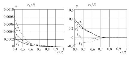
**Fig. 2.** Distribution of the rotation angle in dependence on the radius under rotation of the internal rigid cylinder
