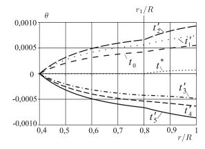
**Fig. 5.** Distribution of the rotation angle in dependence on the radius under the rotation of the external rigid cylinder
