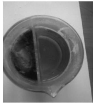
**Fig. 6.** Co-EDTA solution (separated by a diaphragm, with the cathode being on the left) after the electrochemical process.
