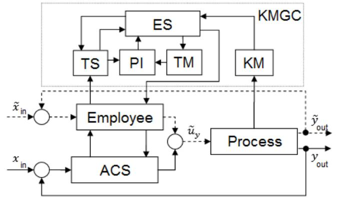
Fig. 1. Man-machine process control system
