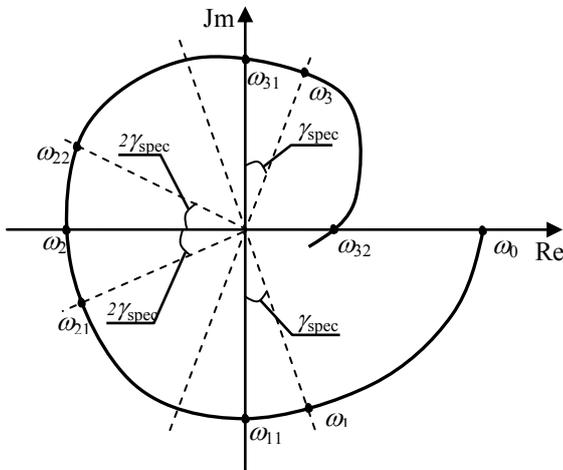
Fig. 2. Expanded frequency response of the control object
